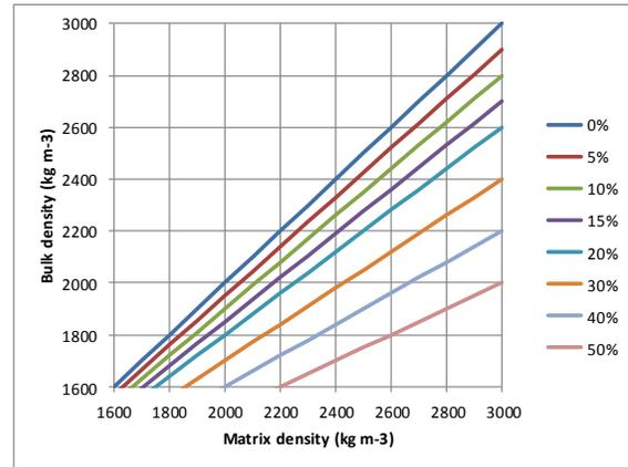
Figure 9: Influence of porosity on the bulk density of a rock. Legend shows the porosity change in percent.
