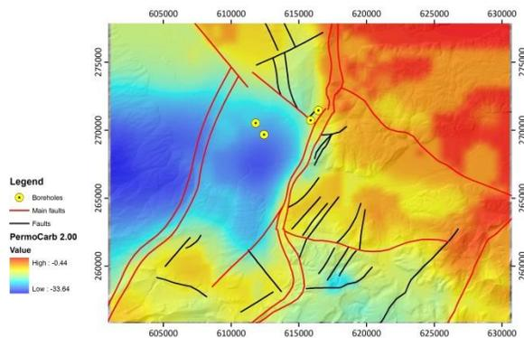
Figure 8: Gravity forward modeling of the 3D geological model including the Permo-Carboniferous sediments below the base of the Mesozoic sediments (Ustaszewski, 2004) with an attributed density of  $2000 \text{ kg m}^{-3}$ .
