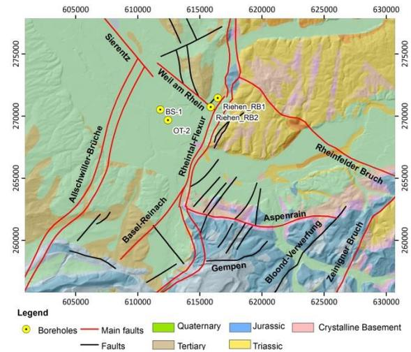
Figure 3: Geological map of the area of the geothermal sites of Riehen with the wells RB1 and RB2 and Basel with the wells BS-1 and OT-2. The fault zones are compiled from different studies (Delacou et al., 2009). Red: major fault zones modeled as fault zones cutting the entire geological model; black: minor fault zones modeled with finite depth extension.
