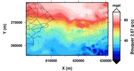
Figure 6: Complete Bouguer anomaly of the area of investigation obtained using GraviFor3D (Abdelfettah and Schill, subm.).
