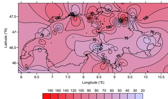
Figure 1: Heat flux map of Switzerland (after <http://www.heatflow.und.edu>) in  $\text{mW m}^{-2}$ . Small black dots: measurement points; open triangles: locations of geothermal wells Otterbach-2, Basel-1, Riehen-1 and Riehen-2; open dots: locations of Bad Zurzach and St. Gallen; black line: outline of the Swiss border.
