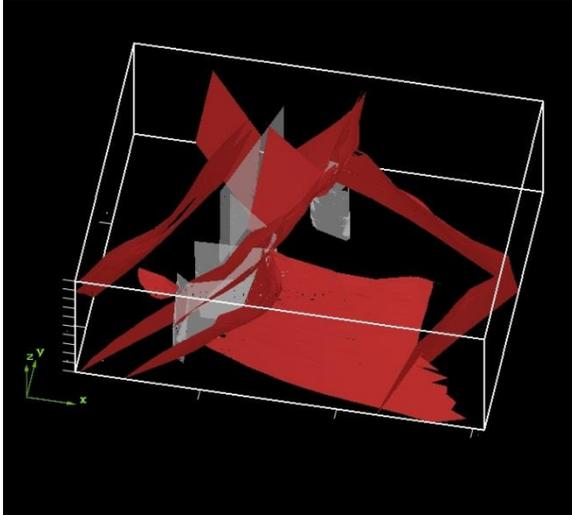
Figure 4: Fault model of the major faults represented in red as infinite faults with constant offset. White planes are used to increase the accuracy of the model. They do not appear in the final model.
