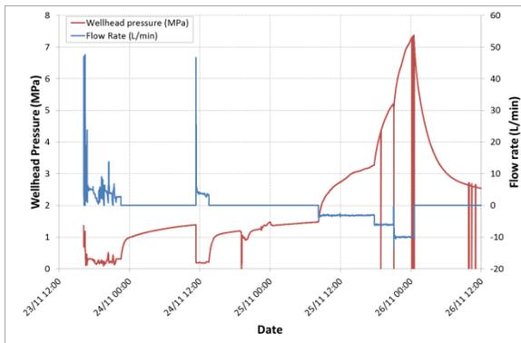
Figure 10: Hydraulic test in the open hole section of the Basel-1 well. The open hole section is located entirely in the crystalline basement over a depth of the open hole section (4629–5000m below surface) containing two major fractures zones.
