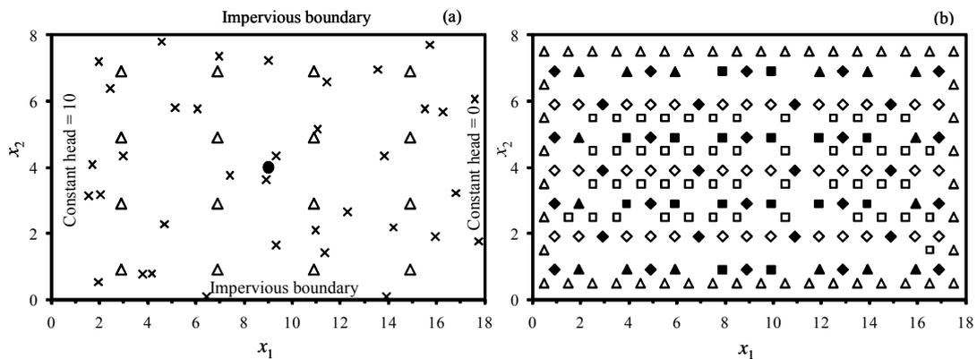
Figure 1: (a) Geometry of the test problem, location of the pumping well (●),  $Y$  (△) and  $h$  (×) measurement points; (b) pilot point locations:  $N_p = 16$  (■),  $N_p = 32$  (■ and ▲),  $N_p = 64$  (■, ▲ and ◆),  $N_p = 103$  (■, ▲, ◆ and ◇),  $N_p = 150$  (■, ▲, ◆, ◇ and △),  $N_p = 200$  (■, ▲, ◆, ◇, △ and □)
