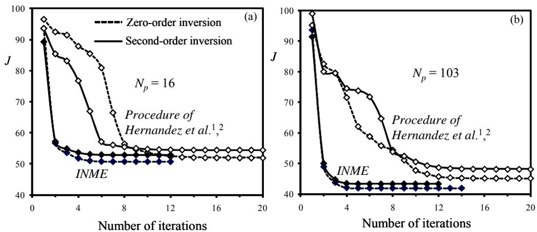
Figure 3: Dependence of  $J$  on the number of iterations for zero- and second order inversions performed with INME ( $\blacklozenge$ ) and with the procedure of Hernandez et al.<sup>1,2</sup> ( $\diamond$ ) with (a)  $N_p = 16$  and  $N_p = 103$
