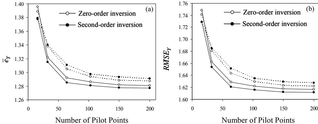
Figure 4: (a) Mean absolute error,  $\bar{e}_Y$ , and (b) root-mean square error,  $RMSE_Y$ , of  $Y$  versus the number of pilot points calculated with zero- and second-order inversion
